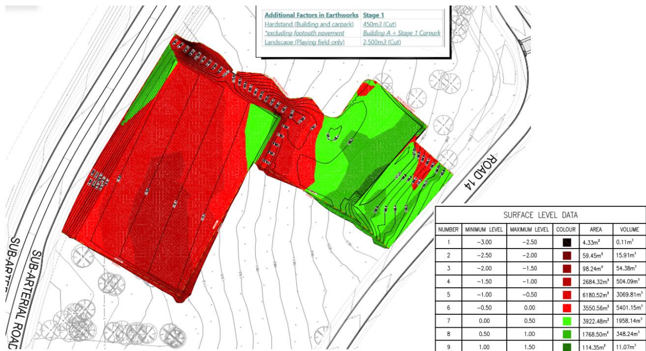
Picture 10 Stage 1 Bulk Earthworks Plan
