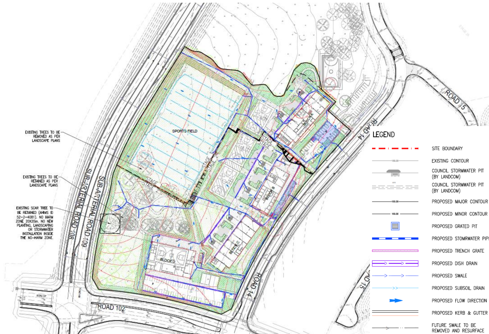
Figure 23 Stormwater General Arrangement Plan
